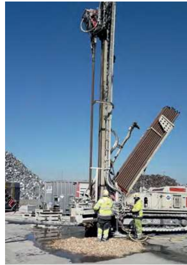
The MC 900P drill rig from Comacchio was operating at the limit of its capability drilling geophone wells with a maximum depth of 1,000m
